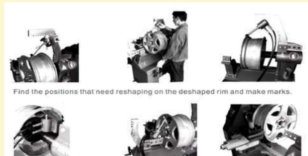
Find the positions that need reshaping on the deformed rim and make marks.
